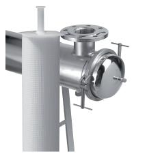
support core. Amazon Filters also offers cartridges manufactured with stainless steel cage and core and nylon end fittings. These are particularly suited for applications where higher temperature ratings are required or compatibility may be an issue. Thermal welding processes seal all components, eliminating adhesives and extractables and optimising cartridge integrity. In-house developments have optimised the pleat pack ensuring rigidity is maintained at all flow rates.
