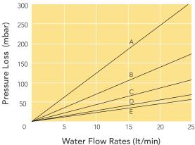
A=0.03µm B=0.1µm C=0.2µm D=0.45µm E=0.65/0.80/1.0µm
