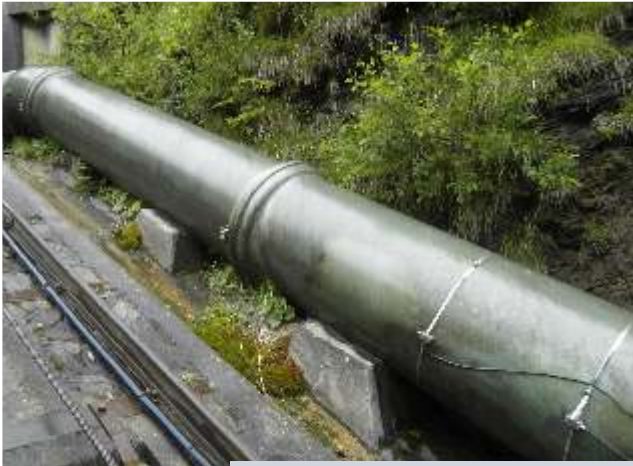
Turbine intake flow measurement using clamp-on sensors
